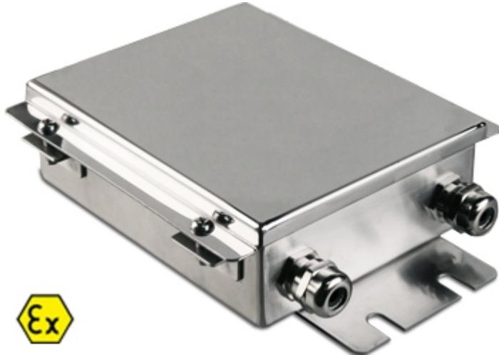
Stainless steel junction box with IP66 protection from water and dust, and fitted with an intrinsically safe electronic board for junction and equalisation of load cells. Terminal boards with screws for easing the connection of the load cells and signal adjustment trimmer, for an accurate and reliable equalisation.
